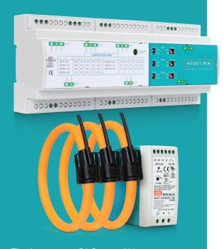
The Accuency 5A Rogowski Integrator Kit (RIK 5A) conveniently provisions up to three channels for Rogowski coils to be integrated to any metering device application that accepts a 5A input. Each integrator channel can be adjusted to accept one of seven field configurable CT ratios for added flexibility. The RIK 5A can be used on services up to 60,000A AC.
