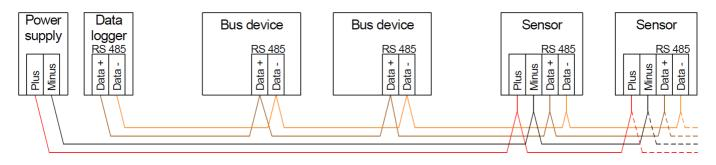
All bus participants with Modbus protocol (RTU) require identical Modbus parameters but different addresses. Bus termination usually not required.
