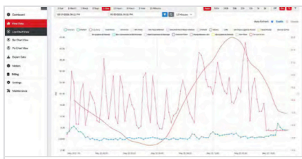
Line chart — per-circuit load with the outside-temperature overlay for direct weather correlation.
